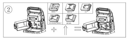
Slide the 18V battery onto the connector until it clicks in place as per diagram 3
