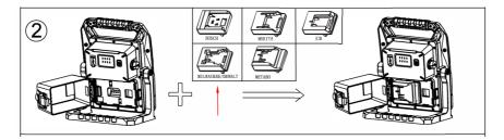
Slide the 18V battery onto the connector until it clicks in place as per diagram 3
